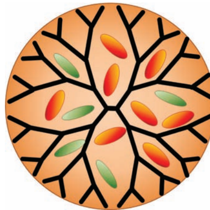
Figure 13. Drawing of a dendrimer carrier encapsulating hydrophobic drug molecules in the dendrimer's voids to increase their aqueous solubility and control their release rate.
